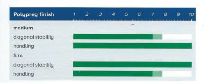
We recommend a **medium** or **firm Polypreg finish** for our **Fibercon® Pro** cloth. The medium Polypreg finish is optimised for ease of handling, and the firm Polypreg finish for the diagonal stability needed in more performance oriented sails.
